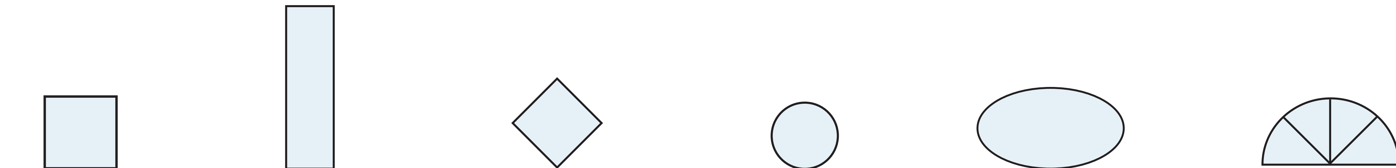
Square Rectangle Diamond Circle Oval Half Moon with or without glazing bars Depending on sash width 245mm x 245mm 175mm x 695mm 245mm x 245mm 245mm x 245mm 492mm x 292mm 382mm x 382mm 175mm x 892mm 382mm x 382mm 382mm x 382mm 642mm x 392mm
